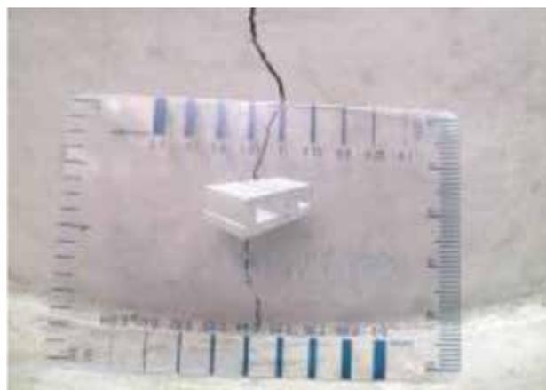
Fig. 3: Typical crack width of 0.04 in. (1 mm) in untreated or SRA-treated concrete specimens
