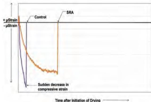
Fig. 2: Sudden decrease in compressive strain at cracking in ring test
