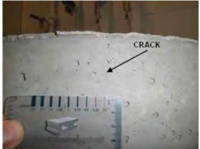
Fig. 5: Typical crack width of 0.004 in. (0.1 mm) in CRA-treated concrete specimens
