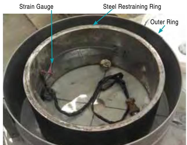
Fig. 1: Ring test setup
