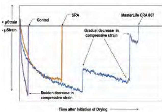
Fig. 4: Typical performance of CRA-treated concrete specimens showing gradual decrease in ring compressive strain compared to sudden decrease in non-CRA-treated specimens
